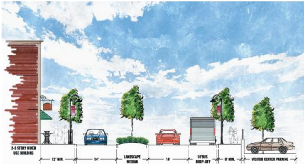
This cross-section shows the dimensional relationship between streetscape components for the proposed boulevard on Franklin Street. The landscape median should be a minimum of 10' wide.
